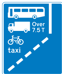
Near-side, with-flow bus lane ahead that can also be used by lorries, pedal cycles and taxis
